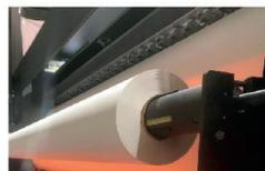
Air shaft feeding and take up bar, ensure heavy paper loading.
